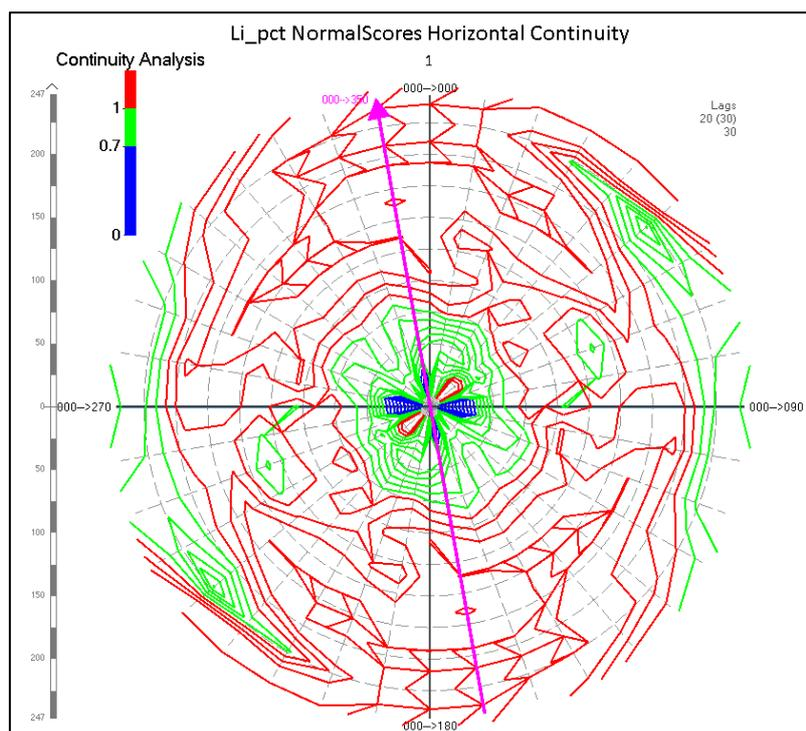
Based on the continuity models, experimental Normal Scores variograms were produced for Li, Sn, and Ta based on the 2 m composites.
